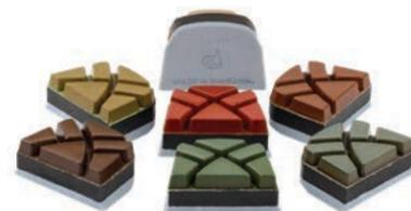
**RECOMMENDED RPM:** for up to 120 grit tools - 650-750 rpm on electric machines; 1800-2100 on propane machines; for 200 grit and up - 800-1100 rpm on electric machines; 2600-3600 rpm on propane machines.
